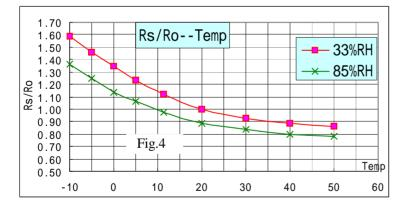
Fig.4 is shows the typical dependence of the MQ-3 on temperature and humidity.
