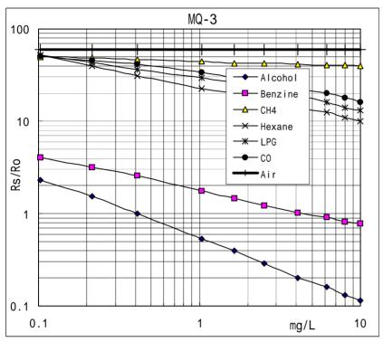
Fig.3 is shows the typical sensitivity characteristics of the MQ-3 for several gases.
